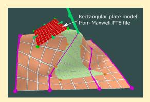
Provus supports rectangular plate modelling. Initiate a plate model or load it from a Maxwell ".pte" file. Manipulate the plate interactively and co-simulate with other plates and/or Provus conductors. Promote a plate to a Provus conductor and begin to deform it into more complex shapes.
